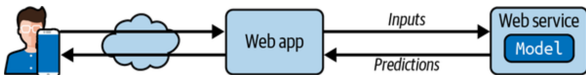
Figure 2-20. A model deployed as a web service and used by a web application
