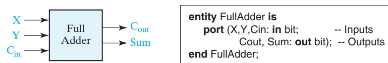
FIGURE 10-10 Entity Declaration for a Full Adder Module
