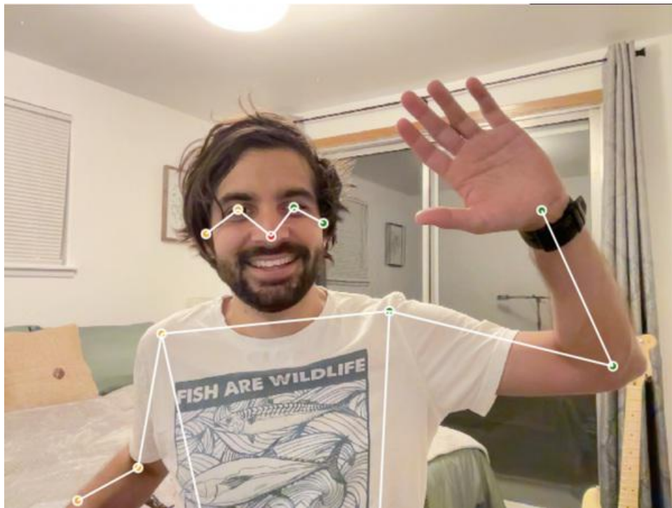
Figure 4-9. Pose estimation identifies key points on a human body, the position of which can be used as input for other processes
