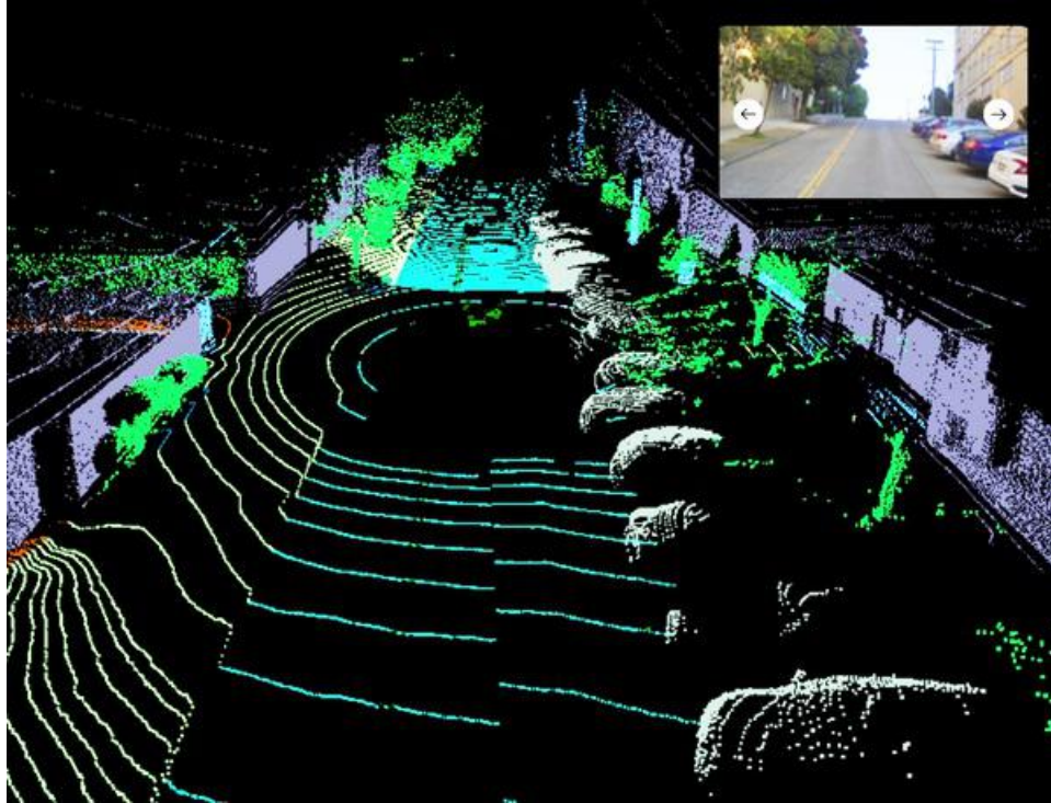
Figure 3-4. This image from the PandaSet open source LIDAR dataset shows a typical LIDAR “point cloud,” with each point in the 3D visualization representing a distance that was measured by the laser; the inset photograph at the top right shows the same scene from the perspective of an image sensor
