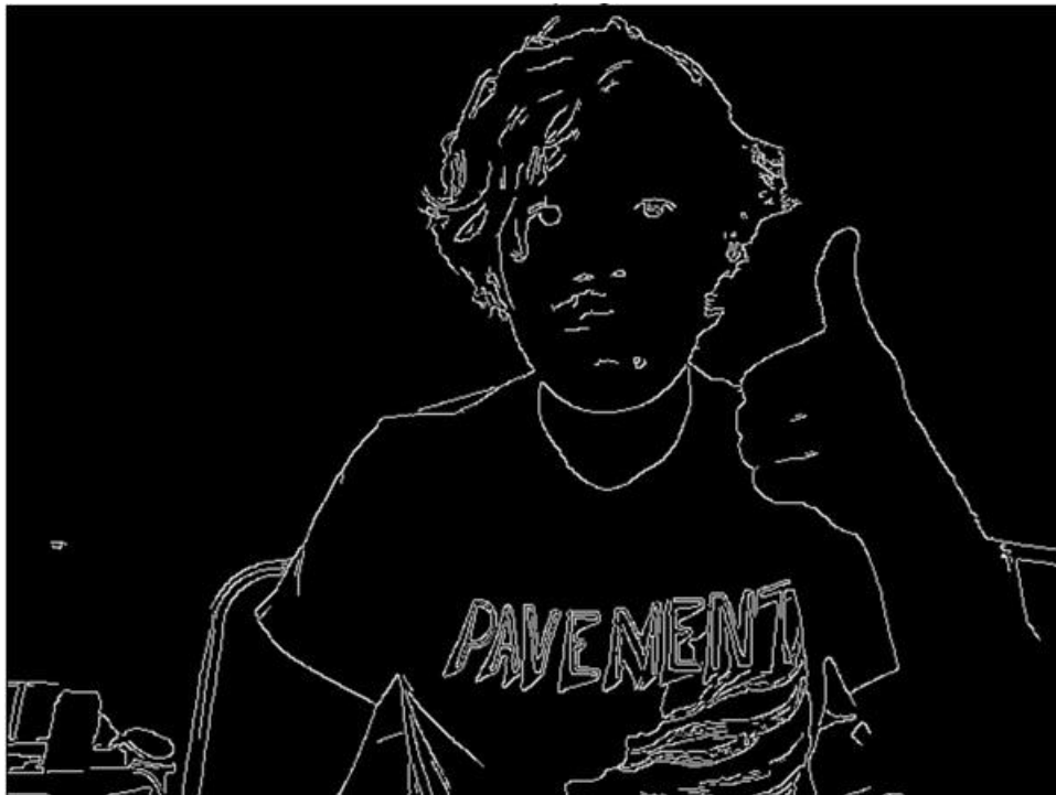
Figure 4-6. Edge detection algorithms find boundaries between areas with different colors or intensities
