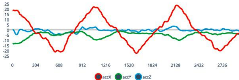
Figure 1-5. The output of a three-axis accelerometer sampled at 6.25 Hz
