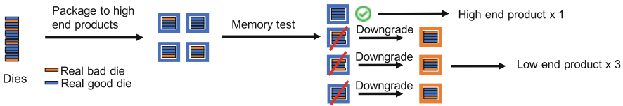
Fig. 6.3 The packaging and memory testing process without a classifier
