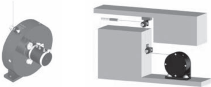
Figure 15.2.4: Pulleys and idlers allow displacement cable to be routed to the application.
