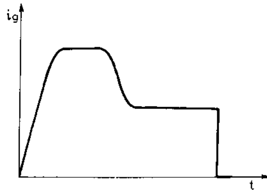
Fig. 4.7. Typical waveform for gate current.
